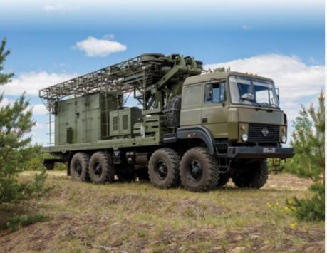
P-18-2 radar is highly mobile and able to receive additional (flight) information from airborne transponders using the integrated secondary radars.
