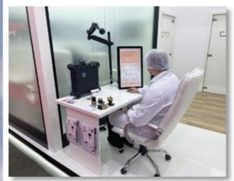
CyberPAS — a personal digital assistant — helps to control manual work in a manufacturing process. The system aggregates the process variables, analyses and makes predictions on the big data basis.
