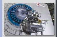
Twenty-five successful starts of the VK-1600V demonstrator engine were performed at the test facility of Rostec United Engine Corporation's ODK-Klimov. The tests continue. An experimental work package was carried out during the tests of VK-1600V demonstrator engine: adjustment of the engine start-up; checking of joint functioning of the units and systems in various modes; assessment of the obtained parameters for compliance with the product specifications.
