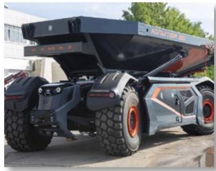
The vehicle is a successor of the KAMAZ line of mining dump trucks. The unmanned vehicle, named Jupiter 30, is designed to transport loosened rock mass or ore using unmanned technology - without the presence of people in the danger zone of heavy vehicles and excavators. Because of this feature, there is no cab for the driver.
