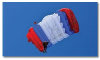
The design of the Malva-24 parachute system with Comfort knapsack ensures reliable operation when the parachute system is put into action at an altitude of 2000m above sea level at a flight speed of 140 to 225 km/h, both with immediate deployment and with delay in
