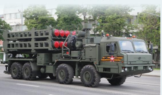
ubai Airshow will see the international debut of the Corporation's S-350E Vityaz SAM system and 98R6E Abakan non-strategic ballistic missile defence system, the latter intended against existing and future tactical and theatre ballistic missiles. The 98R6E comprises the 98L6E multifunctional radar and one or several 51P6E2 launchers. It is a reliable solution against the most dangerous ballistic targets and may be used both independently and as part of air-defence concentrations.
