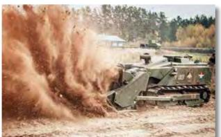
platform. This robotic mine clearer is designed to pass though minefields and demining areas.
