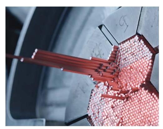
Due to joint efforts of Rosatom State Corporation, TVEL Fuel Company and JSC CMP Russia managed to resurrect unique technologies and implement a project for the industrial production of high-conductive strands for magnetic system of the International Thermonuclear Experimental Reactor being now constructed in France (Cadarache). Competencies gained by domestic companies while performing obligations undertaken by Russia push the boundaries for the development of the national nuclear industry.
